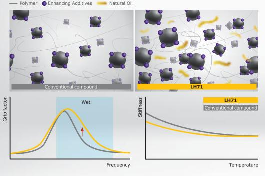
The advanced mixing technology for silica and enhancing additives provides a better wet grip.
